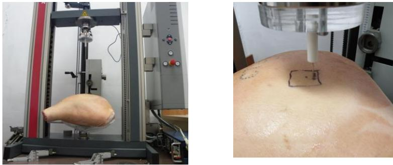
Fig. 6. Tissue resistance on needle insertion experimental setup. Overview on the left; close view on right.
