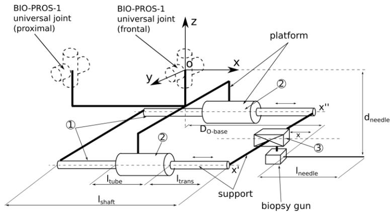
Fig. 4. Conceptual scheme of the needle insertion module
