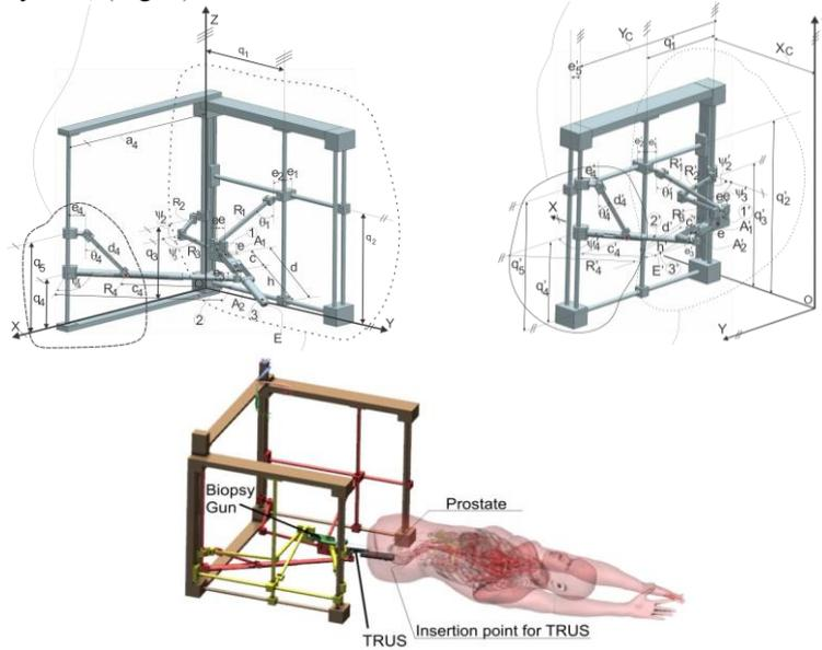
Fig 1. BIO-PROS 1: TRUST guiding module on the top left; needle insertion module on the top right; virtual model within medical environment [15]
