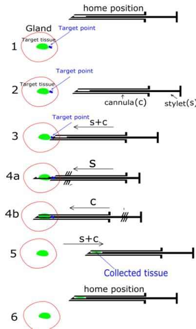
Fig. 2. Protocol for robotic assisted prostate biopsy using a biopsy gun.
