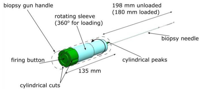
Fig 3. CAD illustration of the biopsy gun.
