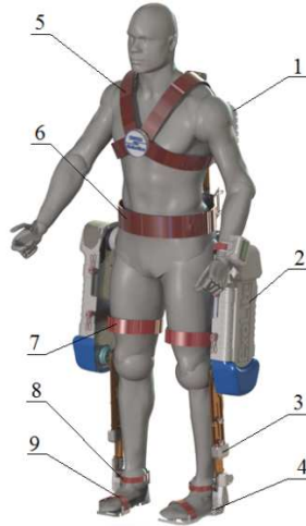
Fig. 1 General view of the exoskeleton (3D model) 1- exoskeleton torso, 2 – thigh link, 3 – shin link, 4 – foot link, 5-9 – connecting belts.
