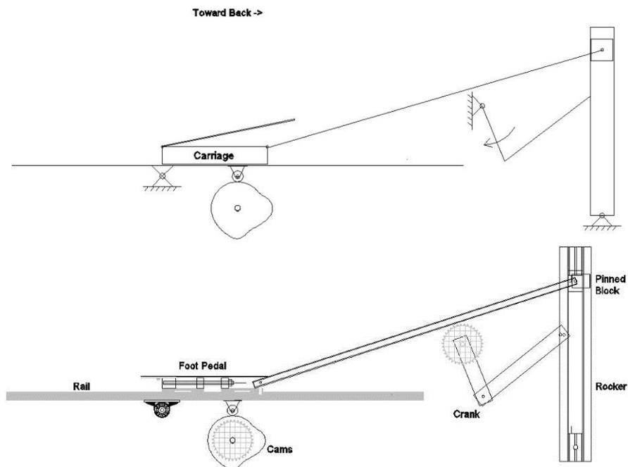
Fig 8 Revised Design Schematic Diagram and Component Models
