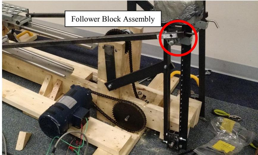
Fig 7 Follower Block Assembly on Crank-Rocker
