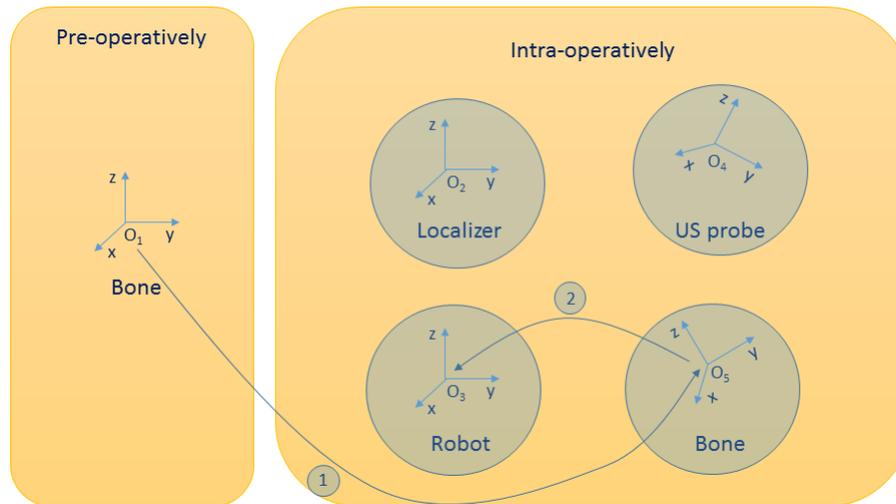
**Fig. 3** Coordinate systems, involved in the navigation system.
