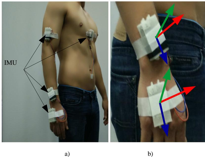
Fig 4. Location of IMU sensors on a testing subject: a) IMUs on the subject body; b) local coordinate system of the IMU
